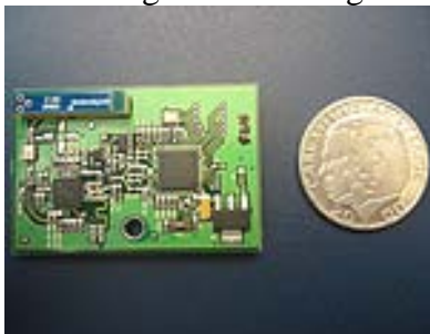
Photograph of the ZigBee module with external power amplifier and low noise amplifier
